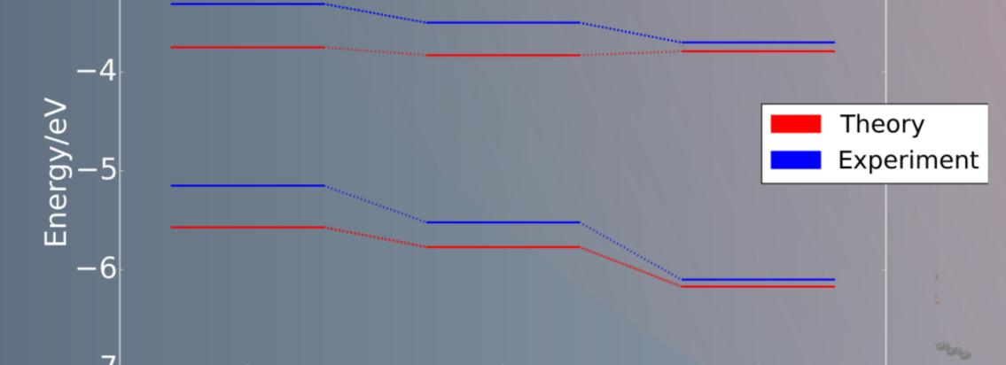
Energy of valence and conduction bands computed for a ternary solar cell composed of two donor polymers (PTB7 and PID2) and one fullerene acceptor (PC71BM). The experimental values (cyclic voltammetry) are taken from Lu, L. et al., Nature Photonics, 8(9), 716-722 (2014).
